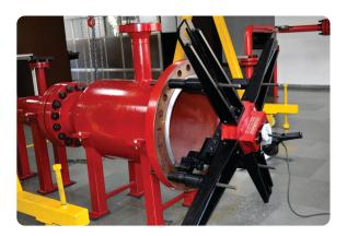
Face Mounted Flange Facer machines are specialized tools used for the maintenance and repair of flanges in pipelines, vessels, and other industrial equipment. Here are some of the key features of external mount flange facing machines.
