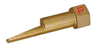
Safe, fast, and effective solution for even the toughest flange alignment jobs. The tool's tapered shaft is a feature that eliminates the need for hammering and prying when lining up flange bolt holes. Flange aligning pin are made of steel and surface coated for rust protection and marked with both the bolt hole size and part number for easy identification.
