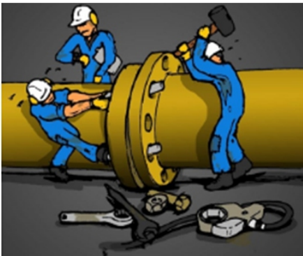
Traditional flange alignment method
