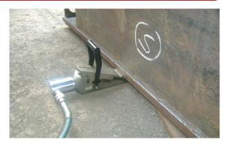
The HVW-10 has been developed as an easy to use / cost effective way to find solutions to heavy lifting where minimal clearance is available. It will lift objects vertically where an access gap of 3/8"(9.5mm) or more is available. The HVW-10 will lift an object fast, secure and safe with a lifting force of 16 Tons per tool. Multiple units can be used if greater lifting force is needed.
