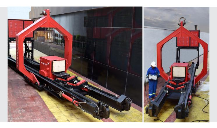
Since the development of the first so called, "bundle pullers" in the late 60's, this successful product has gone through some major changes. Where the first bundle pullers were huge, air driven and slow machines, the new design is all self-contained, easy to operate and slim, making it possible to pull nearly any bundle with minimal effort.
