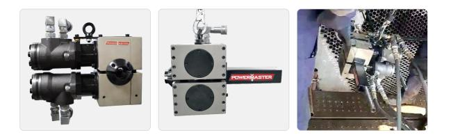
Hydraulic tube spin air is designed to remove Ferrous and Non-Ferrous tubes in round Shape from 5/8" to 1.1 4" OD. Can also be used to extract tubes from 5/8" to 1.1 2" OD using special shaped rolls sized to fit each tube. also, Hydraulic tube Spin air Designed for flatten the Tube with the help of another Gear.
