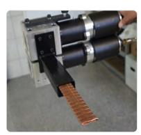
Pneumatic Tube Spinner is designed to remove and flatten non-ferrous tubes from 5/8" to 1.1/4" OD. Can also be used to extract ferrous tubes from 5/8" to 1.1/2" OD using special shaped rolls sized to fit each tube.
